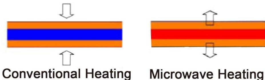
*Fig. 10. Microwave heating (volumetric) versus conventional heating (surface).*
